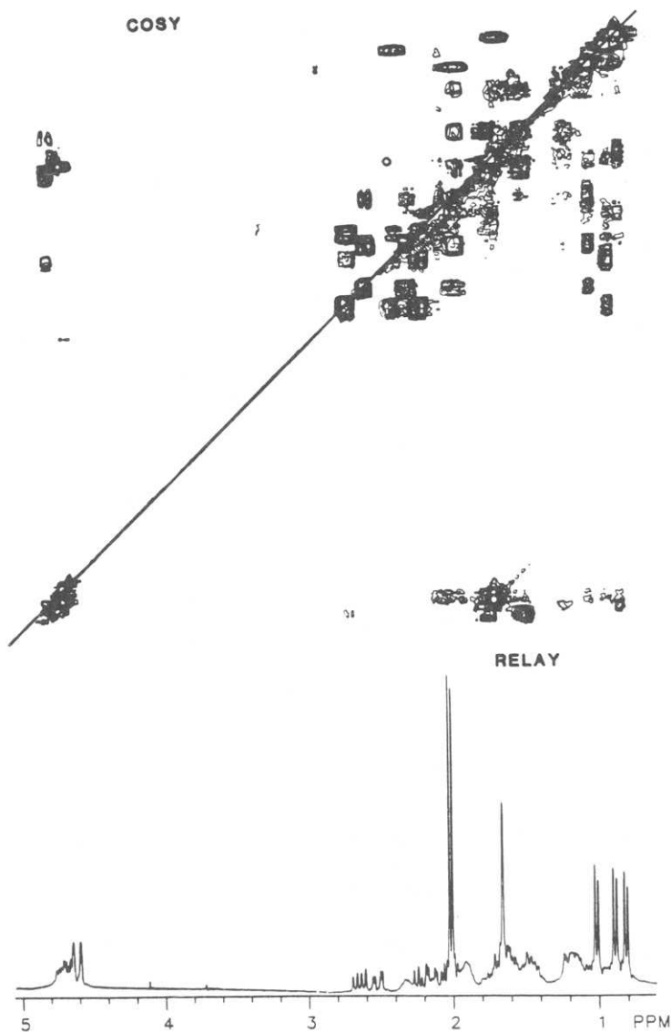
Figure 1. Composite contour plot showing the COSY and RELAY spectra of 3 . The RELAY spectrum shown was optimized for a 3 Hz magnetization transfer ( \tau=1/4J_{HH}=83.3 msec). A second RELAY spectrum (not shown) was also performed using a 5 Hz transfer ( \tau=50 msec) and was necessary to complete the structure elucidation because of the similarities of a number of the proton chemical shifts in the structural fragment shown by 6 .
